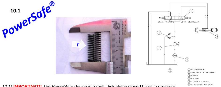
10.1) **IMPORTANT!!** The PowerSafe device is a multi disk clutch closed by oil in pressure.
