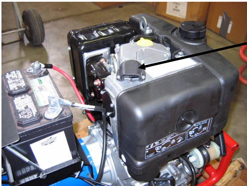
Engine on tractor with battery. Air intake is black "snout".
