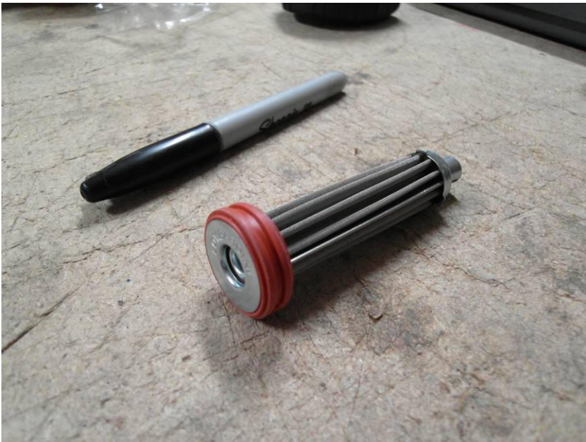
Diesel engine oil filter. Part number: 2175.155. Remember, it is cleanable and reusable. (See instructions on previous page)
