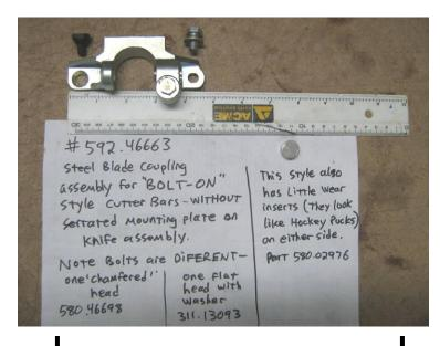
THIS ABOVE BLADE COUPLING DOES NOT USE A SERRATED PLATE. THE BOLT HOLES ARE DRILLED & TAPPED DIRECTLY INTO THE BLADE STRIP, AS SEEN IN THE PICTURE.
