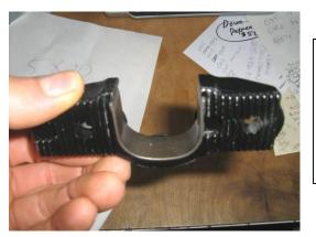
PICTURE SHOWING "SERRATIONS" ON UNDERSIDE OF A BLADE COUPLER
