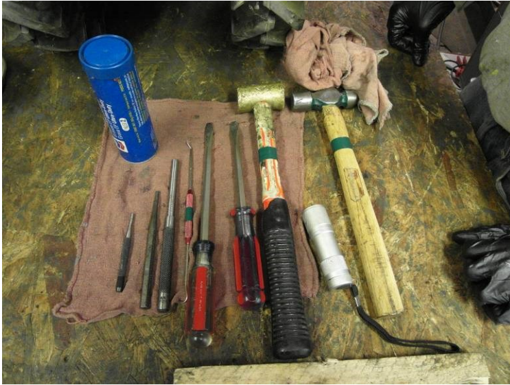
Tools needed for job (3/16" pin punch, screwdrivers, hammer [brass or steel], pick, grease) (you don't need the flashlight...)
