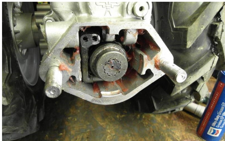
11) Reinstall inner PTO shift lever into PTO flange, aligning bottom "bar" of the lever inside the slot on the coupler.
