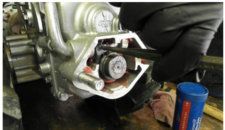
3) Drive roll pins through shift lever with 3/16" straight punch. The pins will fall through the other side into a recess in the housing, and can be easily retrieved after linkage is removed.
