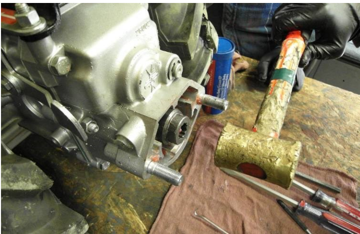
10) Line up holes on PTO coupler with the ball in the PTO shaft, press the coupler into place so that the taper on the rear of the coupler holds the ball down into place, and while pressing in firmly, tap the coupler onto the shaft fully with a soft hammer or piece of wood. (this picture was actually taken a second too late...the coupler is already back on the shaft to the first hole. This is a tricky procedure, and it may take a few tries to get it on.)
