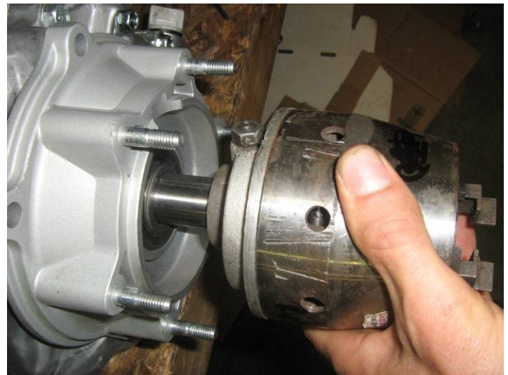
#4. REMOVE CLUTCH FROM ENGINE SHAFT
