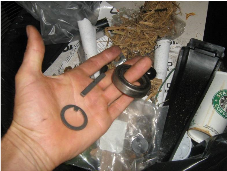
#11. DISCARD OR RECYCLE BEARING, KEY AND THRUST WASHER (NOT NEEDED FOR NEW STYLE CLUTCH)
