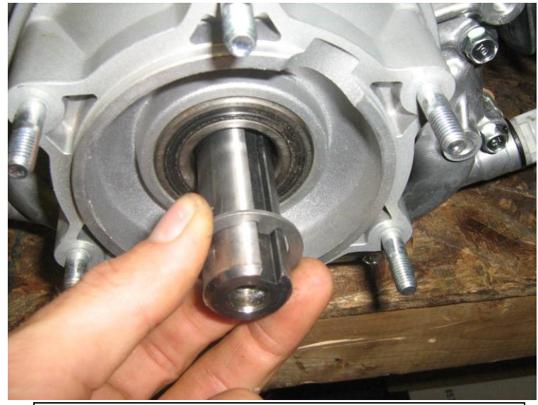
#6. REMOVE THRUST WASHER FROM CRANKSHAFT
