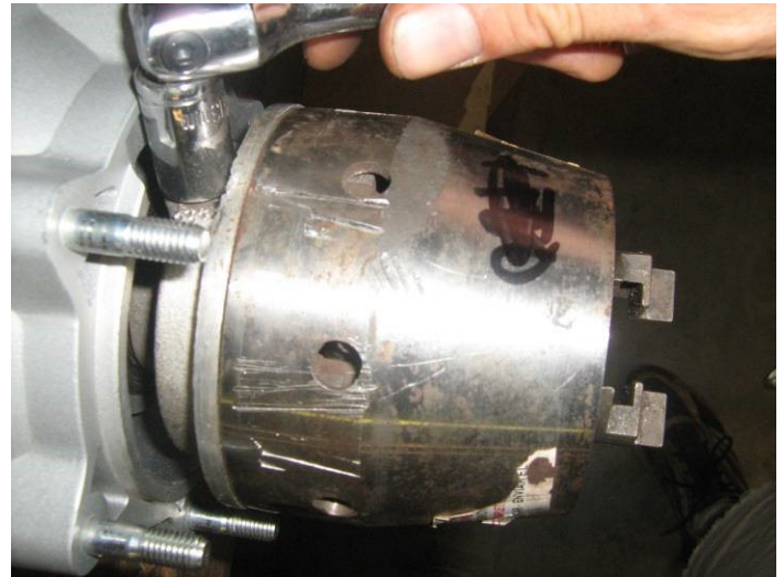
#2. LOOSEN JAM-NUT WITH 13MM SOCKET
