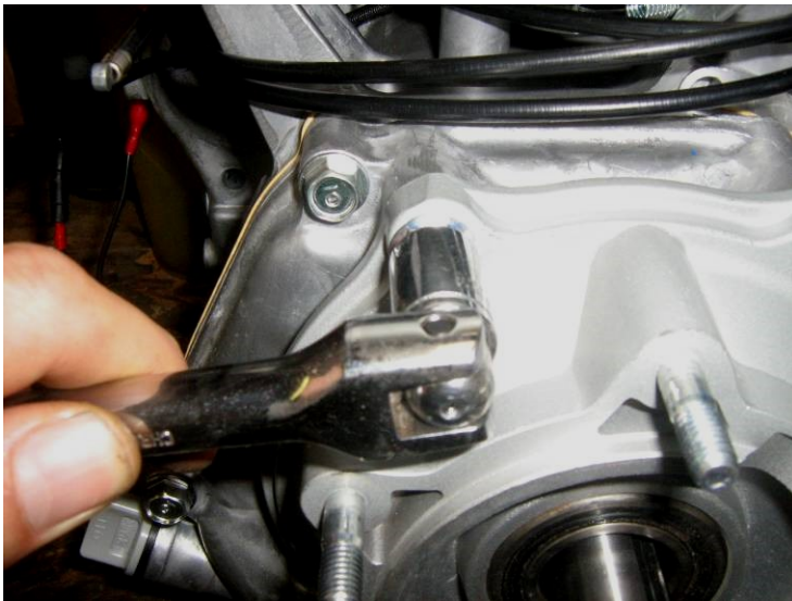
#7. REMOVE QTY. 4 BOLTS HOLDING ENGINE MOUNTING FLANGE TO ENGINE (9/16")
