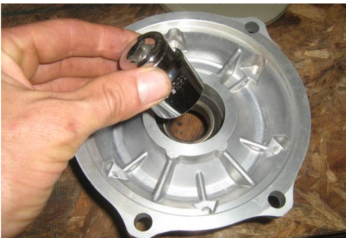
#9. SELECT PIECE OF PIPE, SOCKET, ETC. TO FIT IN BACK OF ENGINE MOUNTING FLANGE, UP AGAINST THRUST BEARING
