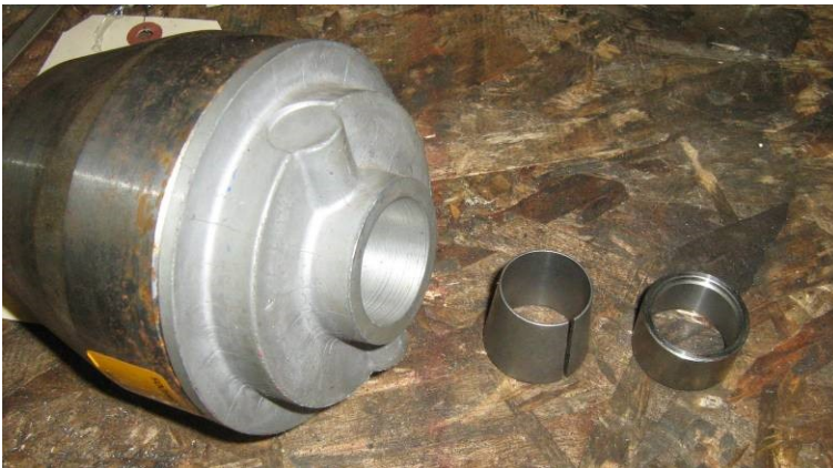
#13. NEW STYLE CLUTCH INCLUDES (FROM LEFT): CLUTCH, SPLIT TAPER-LOCK BUSHING, AND SPACER. MAY ALSO INCLUDE AN ALLEN WRENCH.
