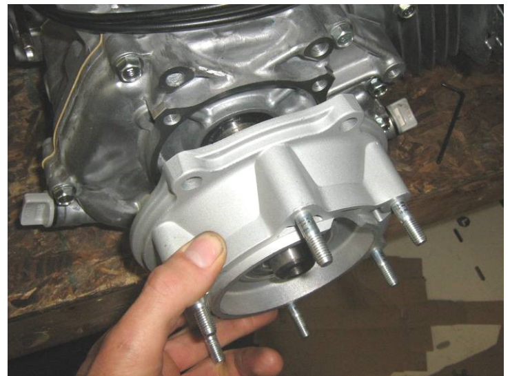
#8. REMOVE ENGINE MOUNTING FLANGE FROM ENGINE
