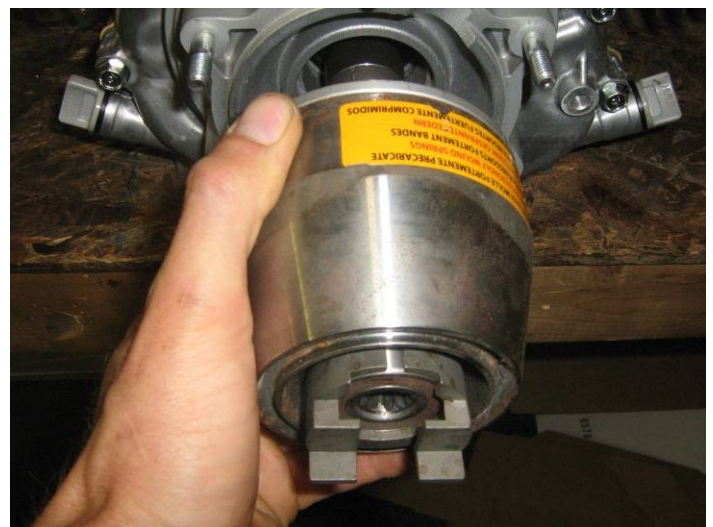
#16. SLIDE NEW CLUTCH ONTO ENGINE CRANKSHAFT
