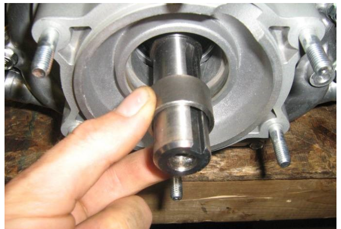
#14. SLIDE SPACER ONTO ENGINE CRANKSHAFT
