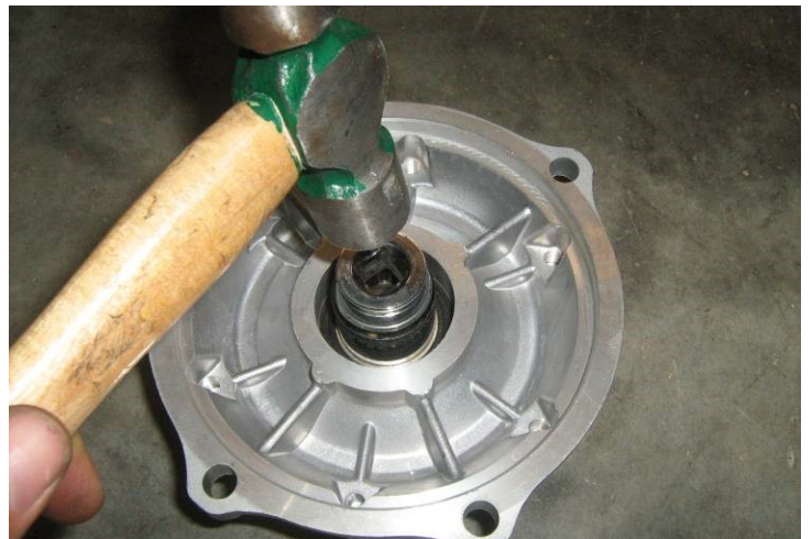
#10. DRIVE BEARING OUT OF ENGINE MOUNTING FLANGE
