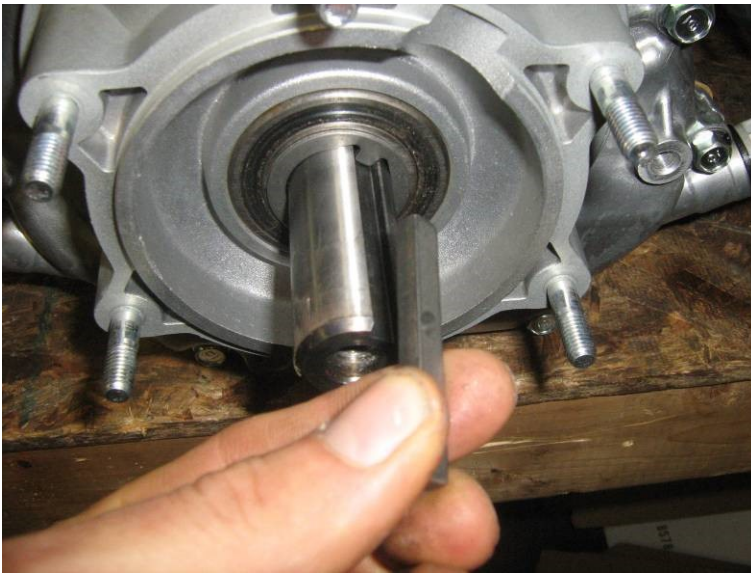
#5. REMOVE KEY FROM CRANKSHAFT
